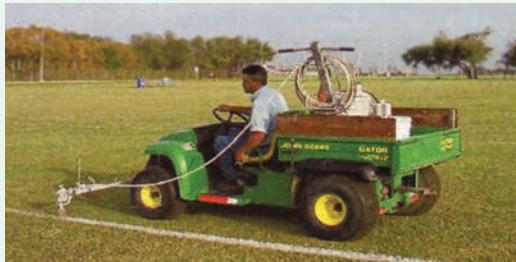
They recycled the metal push bumper of a scrapped vehicle to serve as the front anchor point for the nozzle bar. The spray machine is mounted in the rear compartment. A growth inhibitor mixed with the paint extends the time between markings to every other week.
